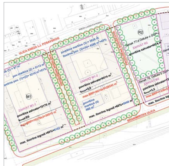
Urban development plan of the area delimited by Lj. Posavskog-Zavrtnica-Branimirova-C. Križa streets in Zagreb
